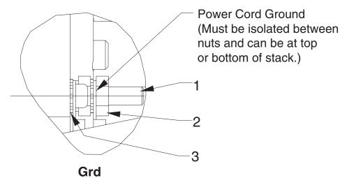
Note: Serrated lockwasher must be adjacent to pump body.
