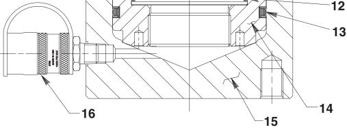
Max. Capacity: 103.1 Tons At 10,000 PSI
